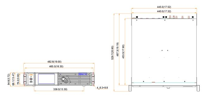
Tolerance: ±0.5 Unit: mm
